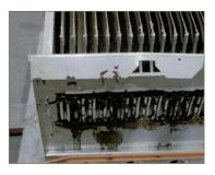
Carrier uses a plastic-coated secondary heat exchanger
